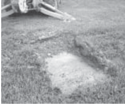
1 st test hole dug in 1" of water, dry soils immediately below surface
